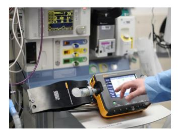
The VT900A Gas Flow Analyzer provides the highest accuracy for testing gas flow and respiratory medical equipment.
